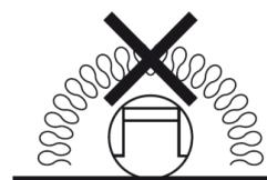
The power supply that can be used where normally flammable materials. Including building insulation, are or may be present, but cannot be abutted against any material and cannot be covered in normal. Minimum clearance distance from the top and sides of the control gear to normally flammable building element is 75mm; as shown in below picture, A=B=C=Min.75mm.
