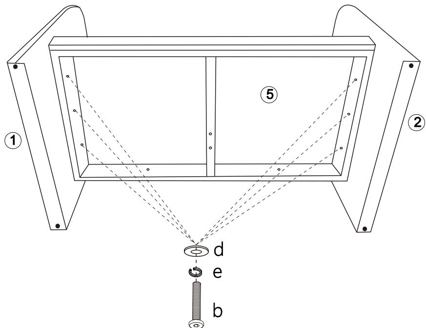
Assemble the handrests first, be careful not to tighten all the screws.
