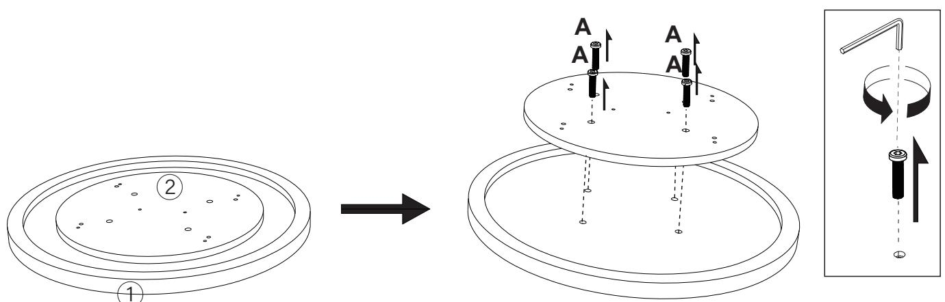
**Components 1 and 2 are pre-assembled and need to be separated first.**
