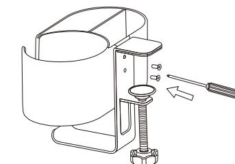
Use a cross screwdriver to lock the screws.
