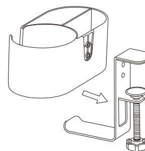
Align the storage box with the positioning screw holes of the support.
