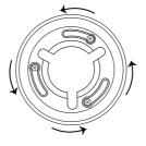
**STEP4:** align the base with the screw position and rotate,make sure the base is securely attached.
