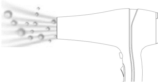
When you use the hair dryer, ions will be produced and released by the air flow.
