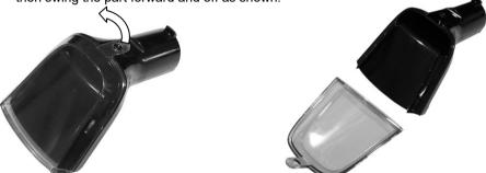
Wash both parts, and the Brushes in warm water (40°C or less) with mild dishwashing detergent then rinse in clean cold water and allow too completely dry.
