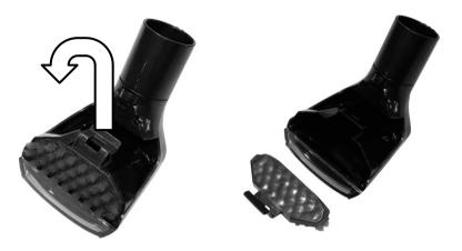
To fit the Silicone Brush or the Bristle Brush, locate the long edge into the floor head then rotate the brush back and push down hard until the latch locks in place.
