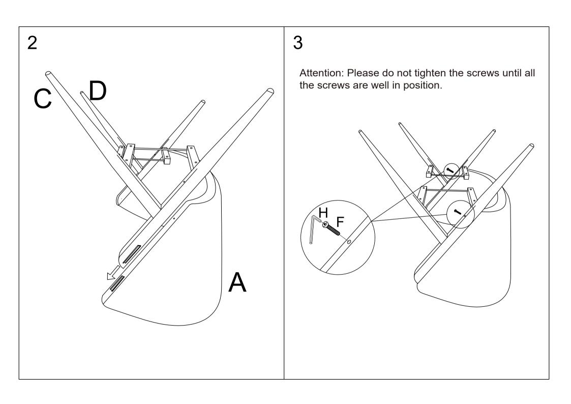
Attention: Assemble screws after the holes of legs and seat bottom alligned. Do not tighten screws until all the screws are well in position.
