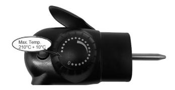
NOTE: When turning the temperature control knob clockwise, each dot point will increase the temperature by approximately 10°C up to a maximum temperature of 210°C.
