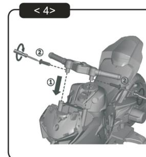
4. Position handle bars into place as shown above and use M4 x 12 screws to secure each side into position.
