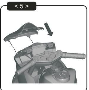
5. Snap windshield into place as shown above. No screws needed.
