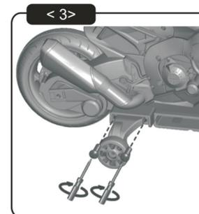
3. Secure side wheels into place using M4 x 12 screws on right side.
