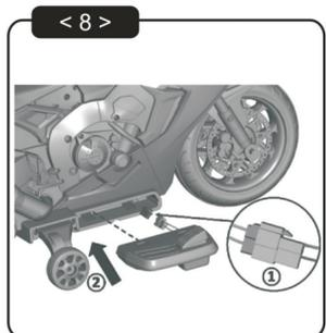
8. Clip the battery connectors into place. Then insert right side tread with foot throttle pedal on it to secure into position.
