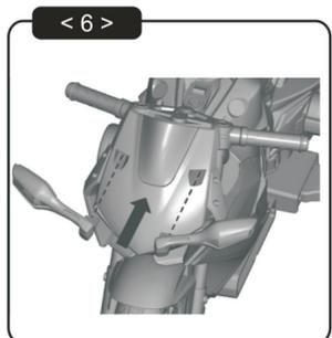
6. Insert left and right rear-view mirrors into place. No screws needed.
