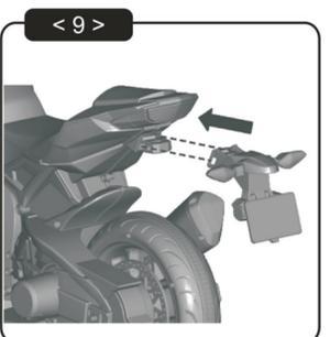
9. Insert tail component into place. No screws needed.
