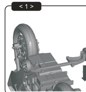
1. Position side wheels into place onto bottom of body.
