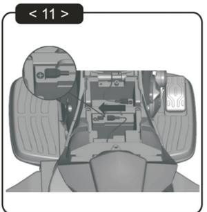
11. Connect red terminal in battery compartment.
