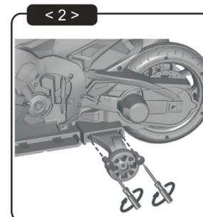
2. Secure side wheels into place using M4 x 12 screws on left side.
