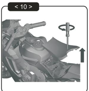
10. Remove seat to access battery compartment.
