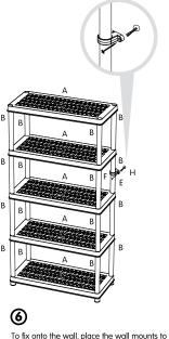
To fix onto the wall, place the wall mounts to the pillars of the shelf. Screw wall anchors into place. Then, insert the screw and tighten.
