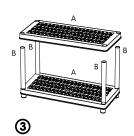
Place another shelf onto the pillars, and ensure the shelf is fully engaged by pressing firmly.
