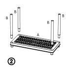
Turn over selected shelf and insert 4 pillars. Press firmly to ensure each pillar is secure
