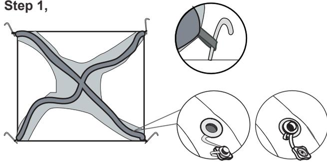
Spread out the inflatable shelter flat, Secure the four corners with nails, Screw on the vent nozzle.
