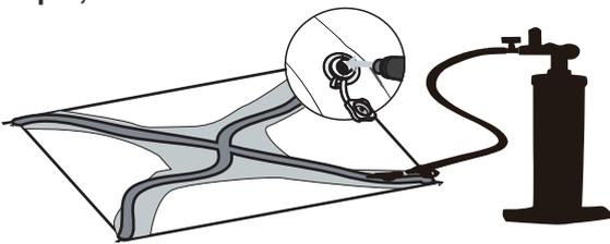
Install the inflatable nozzle on the inflatable shelter, Manual pump rod hard.
