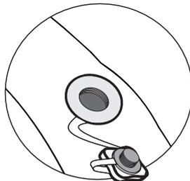
Unscrew the inflator nozzle, roll up the inflatable shelter.
