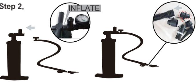
Assemble the tube on the pump body, and Assemble the inflatable nozzle.
