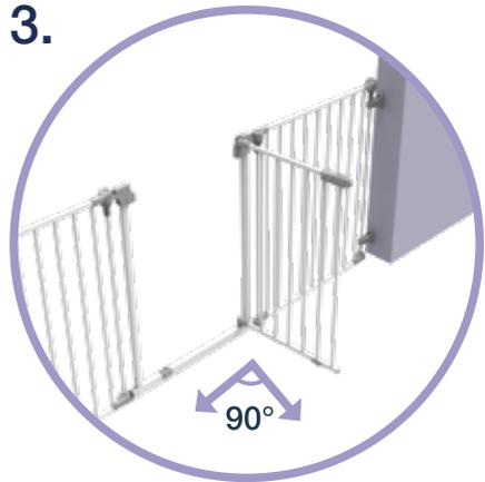
To enable stay open feature, open gate to 90° angle.
