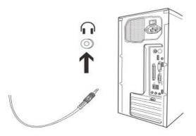
As shown, it is recommended that headphone audio connector be inserted into the headphone holes behind the chassis. The front interface may not be able to output normally due to main board reasons.
