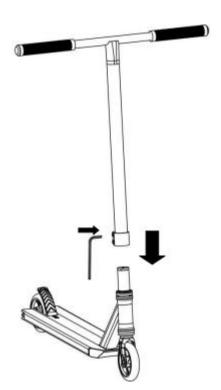
1. Loosen the clamp on steering tube. Slide the tube onto the fork until it is touching the fork headset washers.
