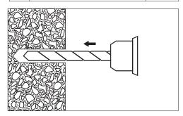
**Step 1:** PART A-screw size:M4,use a drill bit with the same diameter as PART A for drilling.
