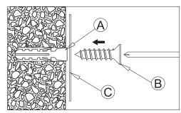
**Step 3:** Screw PART B and PART C into PART A
