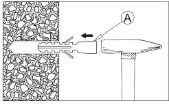
**Step 2:** Insert PART A into the hole
