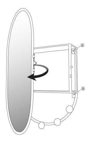
Pull the right border of the mirror frame outward and turn it to where you want it to be. Note: The maximum rotation Angle of the mirror frame is 90 degrees!
