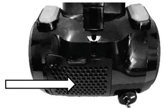
Remove the grill by pushing the top clip downward to unlatch it and then swing it open to expose the filter. (1)
