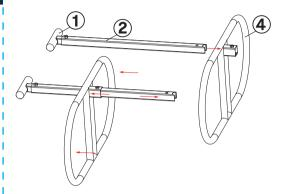
Insert the handle into the support pillar. Ensure that the support pillar passes through the bowl holder.
