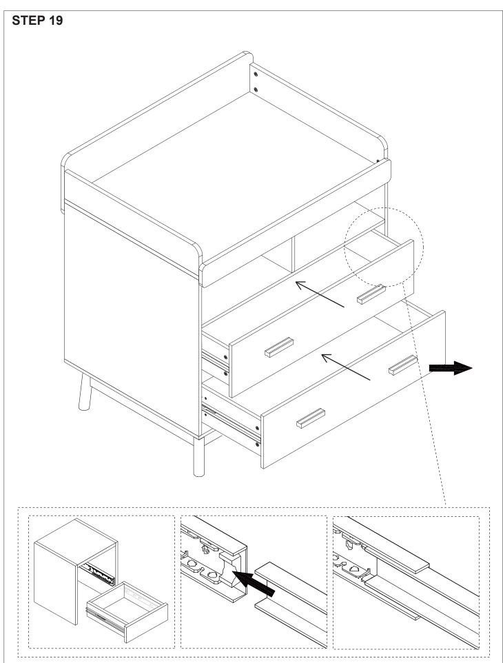
Install the inner fixing rail to the drawer and lock the middle fixing rail in order to allow the drawer to slide open and closed.
