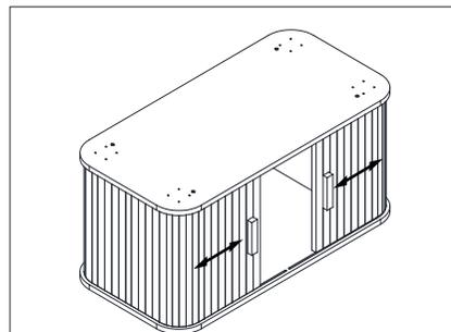
**Attention:** Pls ensure the slider door is in the groove and move door back & forth smoothly before fully screwing.
