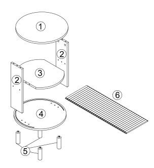
Do not tighten the screws fully during assembly. Fully tighten screws after the final assembly steps.
