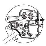
You can adjust one or both hinges on each door, depending on how much correction it needs. If the door seems to be tilting down to the right, turn the side-to-side screw on the top hinge so the hinge pulls closer to the side of the cabinet box, moving the top of the door to the left.
