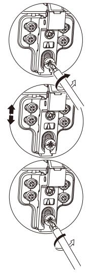
If the door doesn't meet the box at the top, adjust the top hinge toward the cabinet and/or adjust the bottom hinge away from the cabinet. If the door is gapped at the bottom, do the reverse.
