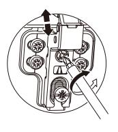
You can adjust one or both hinges on each door, depending on how much correction it needs. If the door seems to be tilting down to the right, turn the side-to-side screw on the top hinge so the hinge pulls closer to the side of the cabinet box, moving the top of the door to the left
