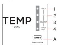
The temperature controls are located on the inside of the fridge. Use the SETTING button (A) to cycle through the temperature settings from COLD (1) to SUPER COOL (4).
