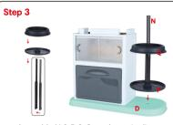
Assemble N & P & Q as shown in diagram, then insert component N into component D as shown in diagram.
