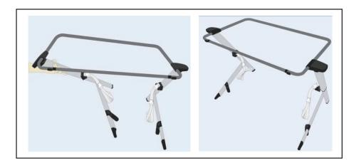
2. Insert the side rail into the middle support frame by lining up the buttons and holes, until you hear a "Click" sound, as shown below.
