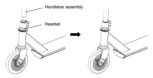
Step 4: Tighten bolts alternately using the allen key provided until secure.
