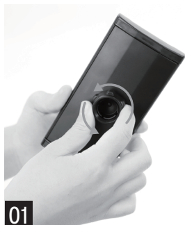
Step 1: Unscrew the nut behind the holder
