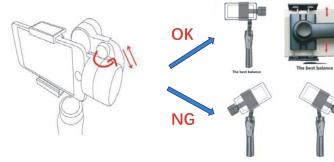
Adjustment methods: Make sure the gimbal switch off before adjust. Load your phone to the bracket. Loose the balance knob and adjustment arm length. The mobile phone should remains at best balance level. Then tight the balance knob.
