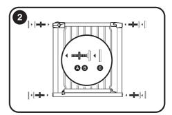
Screw mounting bolts and adjuster screws together and then place into mounting holes in each corner of the gate.
