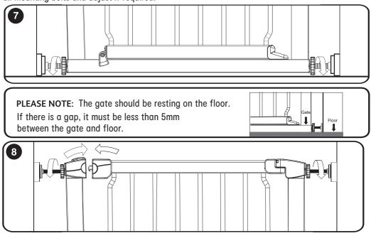
When you unpack the gate, you may notice a gap at the gate opening - this is normal with pressure mounted gates and the gap will disappear when it is installed correctly.
