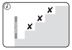
If the safety barrier is used at the top of the stairs, it should not be **positioned below the top level.**
