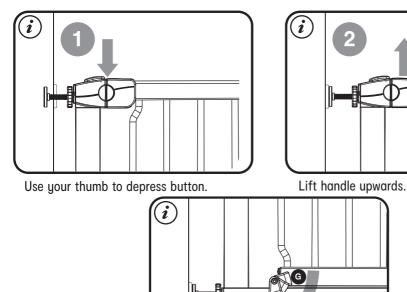
With part G in neutral position, the gate will open in both directions. However when engaging part G, it will act as a stopper and the gate will only be able to open in one direction.
