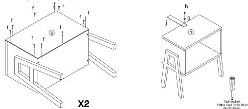
Step 4: Once you use 2 unit stacking Attach anchor fixing j from step 3 onto the wall with a corresponding position. (as per below diagram).
