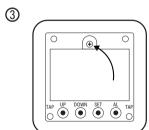
Replace the cover and screw using a screwdriver.
