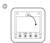
Unscrew the battery compartment to insert batteries.
