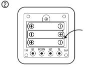
Batteries are to be inserted with the correct polarity.
