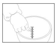
3.Before placing the inner pot into cooker body, check that the pot is dry and free of debris. Place the inner pot into the cooker, turn it slightly from left to right, and ensure the pot is perfectly in contact with the heating plate. Level the rice inside the pot
