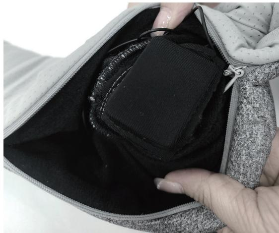
Step 3: Remove the internal controller box ⑥.
