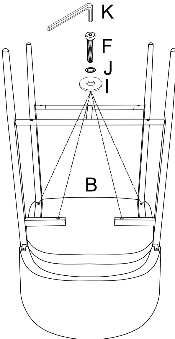
Attention: Assemble screws after the holes of legs and seat bottom aligned.
