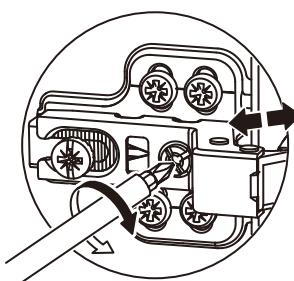
You can adjust one or both hinges on each door, depending on how much correction it needs. If the door seems to be tilting down to the right, turn the side-to-side screw on the top hinge so the hinge pulls closer to the side of the cabinet box, moving the top of the door to the left.
