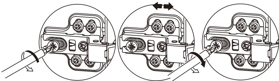
If the door doesn't meet the box at the top, adjust the top hinge toward the cabinet and/or adjust the bottom hinge away from the cabinet. If the door is gapped at the bottom, do the reverse.
