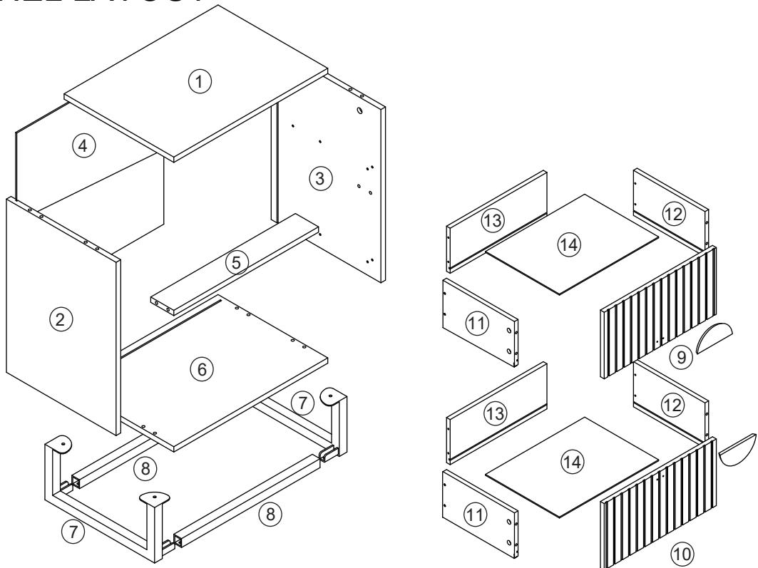
ATTENTION: DO NOT TIGHTEN THE SCREWS FULLY DURING ASSEMBLY. FULLY TIGHTEN SCREWS AFTER THE FINAL ASSEMBLY STEP.
