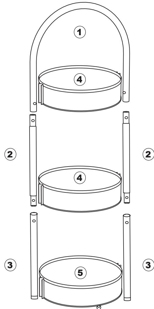
**STEP 1:** Align the holes on the side rods before installing each layer of the basket.
