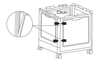
Interlock 4 baffles and press firmly until you hear a click sound
