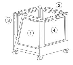
Unlock the baffles and firstly fold the side panel  $\ensuremath{\textcircled{1}}$
