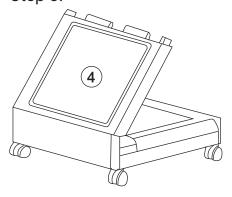
Unlock the baffles and lastly fold the side panel ④
