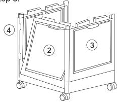
Unlock the baffles and secondly fold the side panel ②
