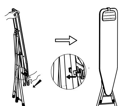
Step①: Release latch, secure support rod to panel bottom
