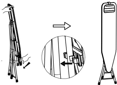
Step①: Slide the centre leg towards the rear of the panel until all legs are aligned
