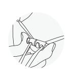
3. Insert the screw into the ball joint.
