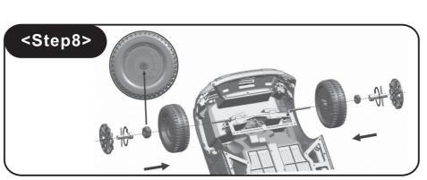
8.Insert the two front wheels and tighten two nuts by the tools provided, cover the wheel caps.
