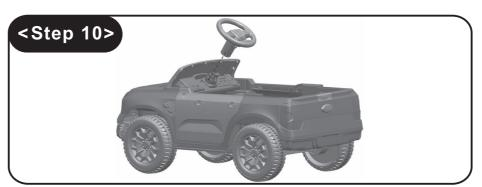
10.Press the button and insert the steering wheel.
