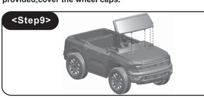
9.Insert the windshield in the front of the body,make sure it is firmly fixed.
