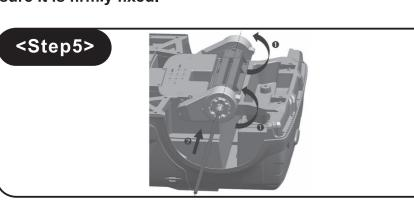
5. Rotate the gearbox and make the hole alignment, then insert the rear wheel axle.
