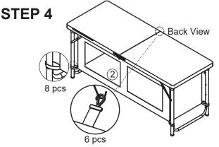
Insert and fasten the storage bag to the frame using all buttons and Velcro straps.
