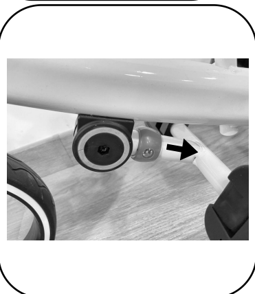
6. Pull the red ring down to fold and unfold the pedal
