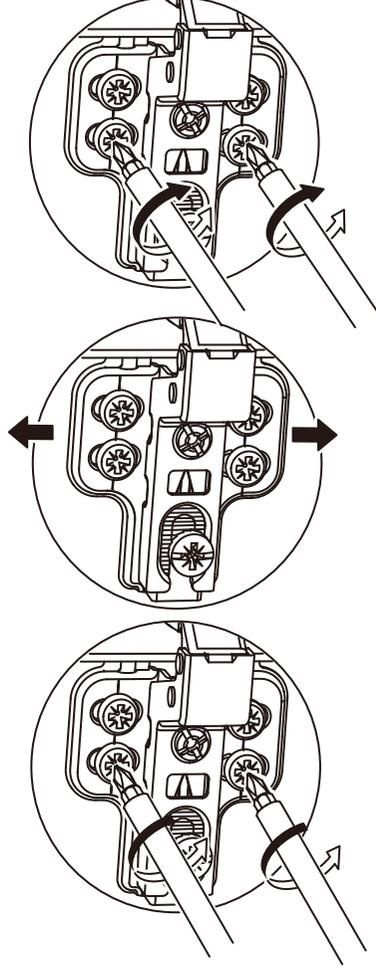
1. Loosen the two mounting screws on both hinges, but only slightly. ...
