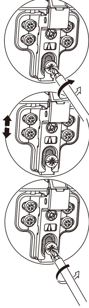
If the door doesn't meet the box at the top, adjust the top hinge toward the cabinet and/or adjust the bottom hinge away from the cabinet. If the door is gapped at the bottom, do the reverse.
