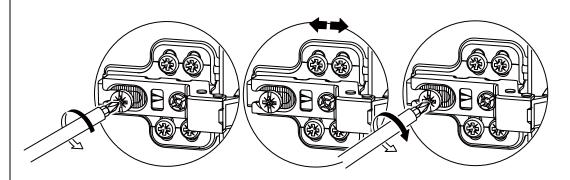
If the door doesn't meet the box at the top, adjust the top hinge toward the cabinet and/or adjust the bottom hinge away from the cabinet. If the door is gapped at the bottom, do the reverse.
