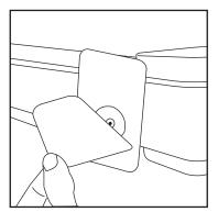
3. Remove the protective film, then stick it to the wall in a straight line. Hold firmly for 30 seconds.
