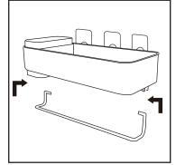
6. Install towel rack on the shelf. After 24 hours, install the shelving to the wall with screws.
