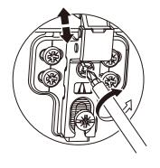
You can adjust one or both hinges on each door, depending on how much correction it needs. If the door seems to be tilting down to the right, turn the side-to-side screw on the top hinge so the hinge pulls closer to the side of the cabinet box, moving the top of the door to the left.
