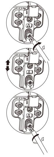
If the door doesn't meet the box at the top, adjust the top hinge toward the cabinet and/or adjust the bottom hinge away from the cabinet. If the door is gapped at the bottom, do the reverse.
