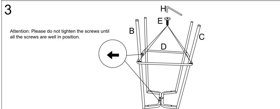
Attention: Assemble screws after the holes of legs and seat bottom alligned.Do not tighten screws until all the screws are well in position.
